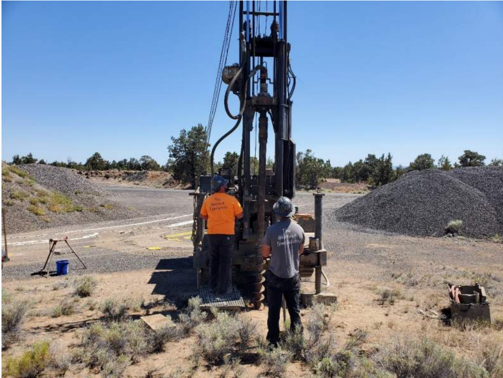
Hollow stem auger flights were advanced until practical refusal.
