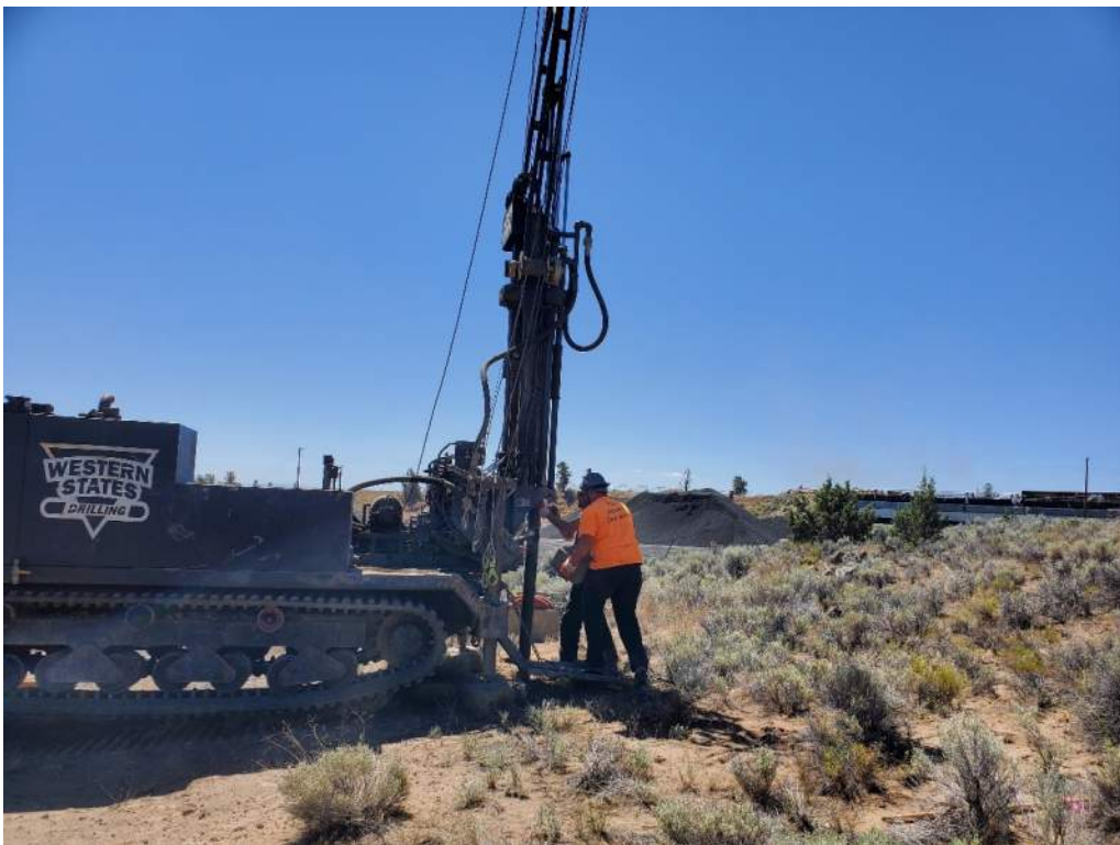
HQ-wireline coring techniques were used to obtain core samples once auger refusal was encountered.
