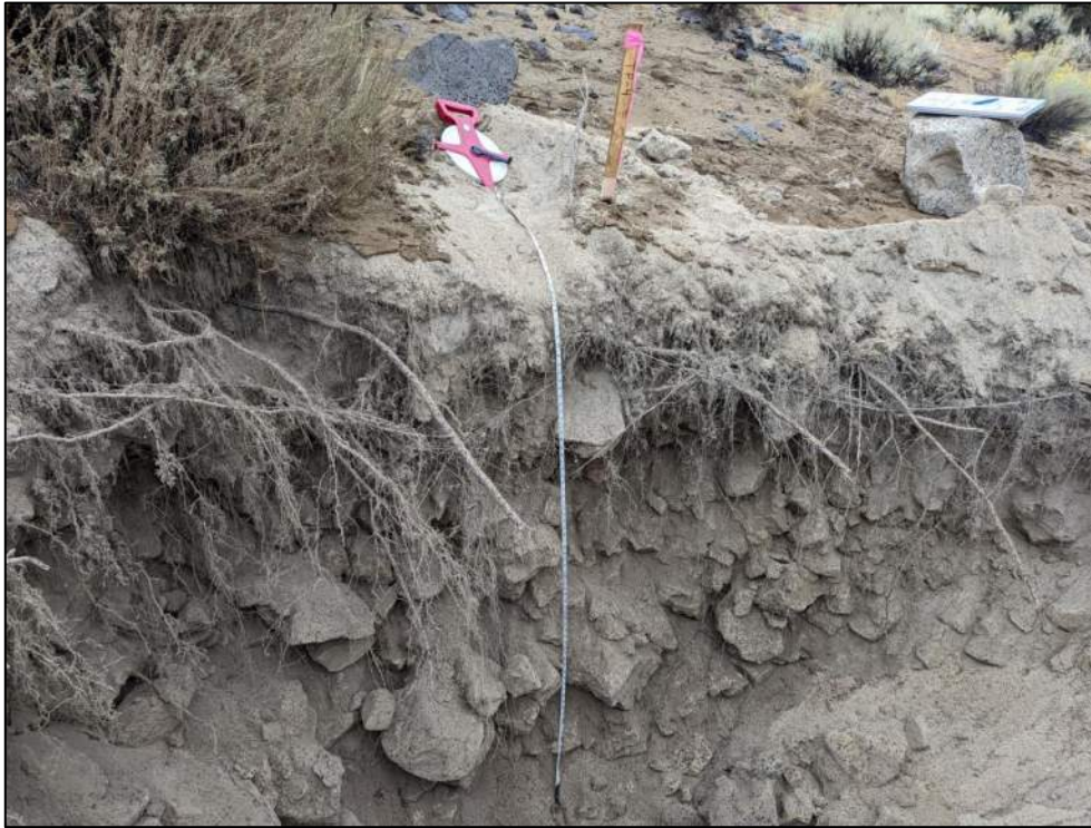
Photo 1. Example of subsurface materials encountered in TP-4. Gravel to cobble materials within a sandy matrix is the upper weathering profile of bedrock.
