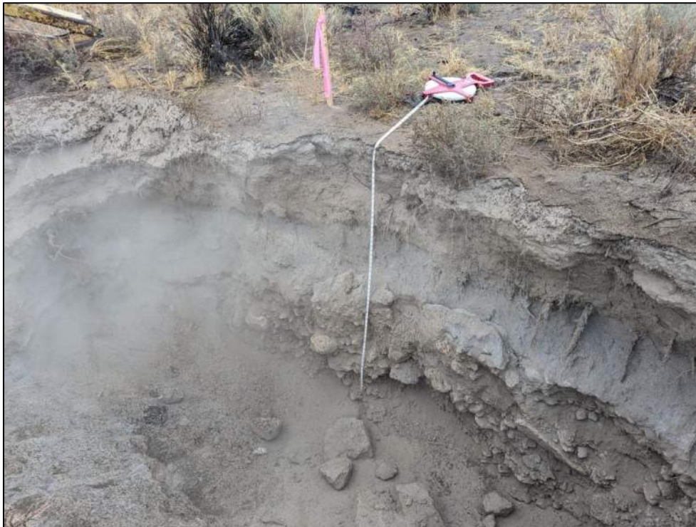
Photo 2. Subsurface materials in TP-5 with more of a well-defined interbed appearance.
