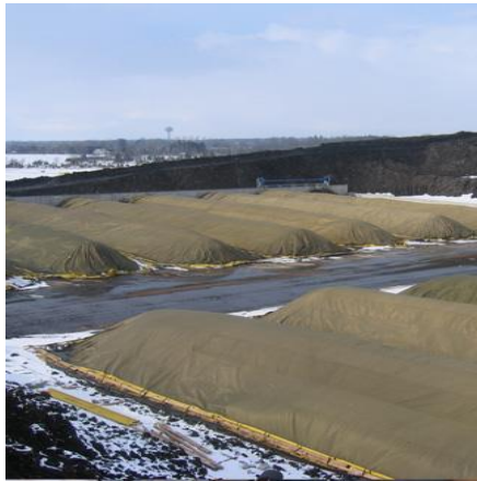
Figure 6-9: Textile covered composting piles-GORE Cover for Organic Waste Treatment (Courtesy of Gore)
