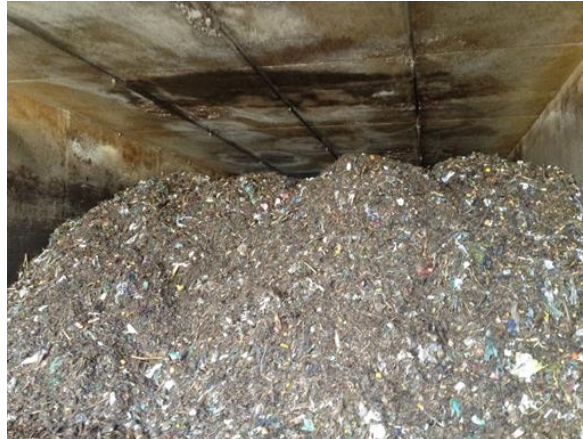
Figure 6-20: Chamber of a High Solids AD with Integral Composting Operation 2 (Images courtesy of Aikan)
