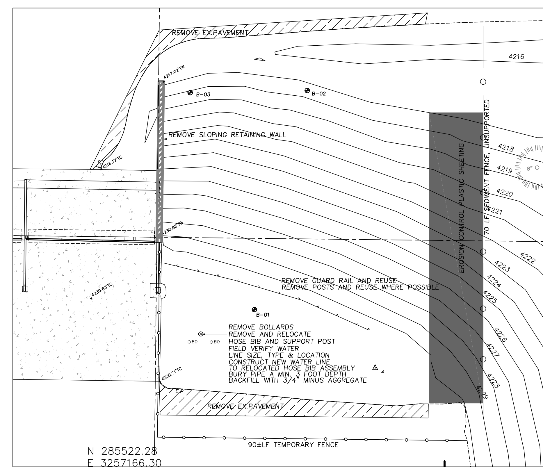
DEMOLITION AND EROSION CONTROL PLAN
