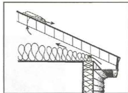
Figure 5.-Passive attic vents.
