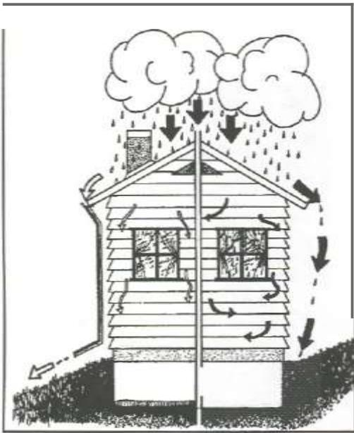
*Figure 1.-Gutters, a slope away from the house, and drainage tile in the foundation keep the left side of this house dry. No gutters, a slope toward the house, and no drainage tile expose the right side to moisture damage.*
