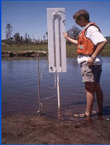
Measuring groundwater level in well
