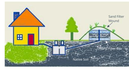
Like a traditional drainfield, bottomless sand filters remove pollutants in the wastewater through biological, physical, and chemical means, although biological activity is the primary treatment process in a sand filter. Sand filters produce high quality effluent, significantly reducing fecal coliform bacteria, removing organics, and nitrifying ammonia.
