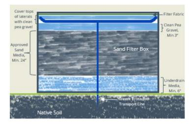
This handout is designed to explain the basic workings of a sand filter system and the basic layout. For construction and material standards for all septic system types refer to Oregon Administrative Rules (OAR) 340, Division 71 and 73,
