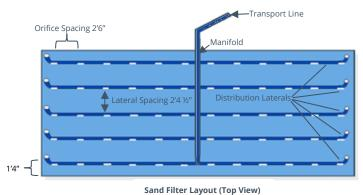
3. Determine the correct pump size to allow for a minimum (5) foot squirt height from the distal orifice in each lateral *with no more than 10% height variation throughout the system.*
