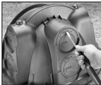
1. Start tear-out seal.
